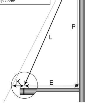
Measure width of sail fitting for mast and boom to nearest 1/16". Circle fitting type and sizes
